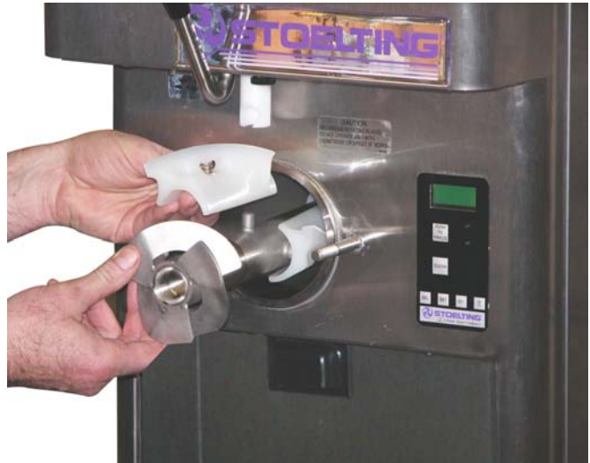
Figure 3-10 Removing Auger Shaft and Flights
