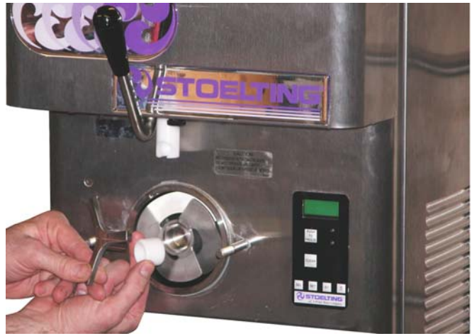
Figure 3-9 Removing Auger Support
