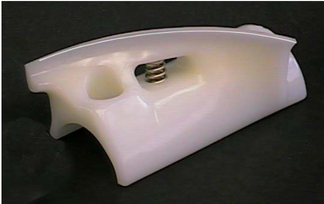
Figure 3-8 Auger Flight Wear
