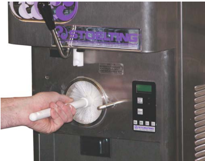
Figure 3-12 Cleaning Freezer Barrel
