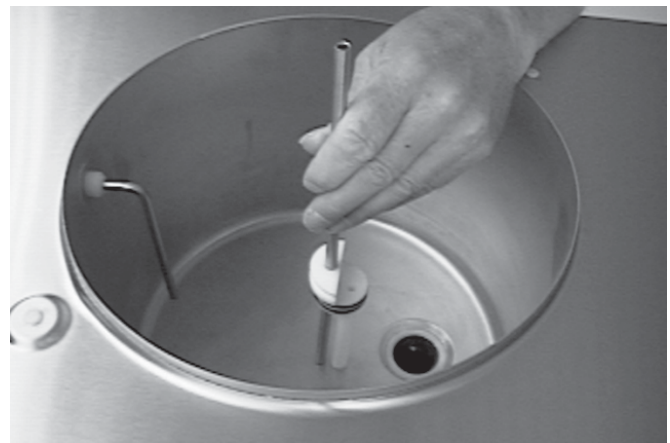
Figure 16. Removing Mix Inlet Regulator
