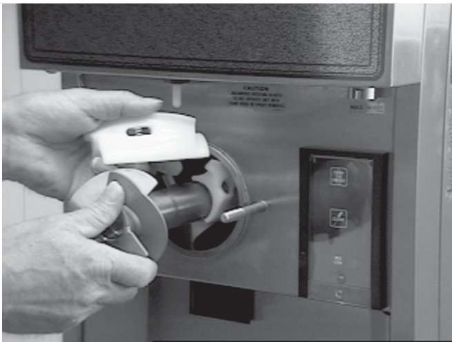
Figure 22. Auger Shaft Removal
